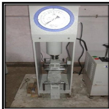
Figure 7: Flexural testing of prism
