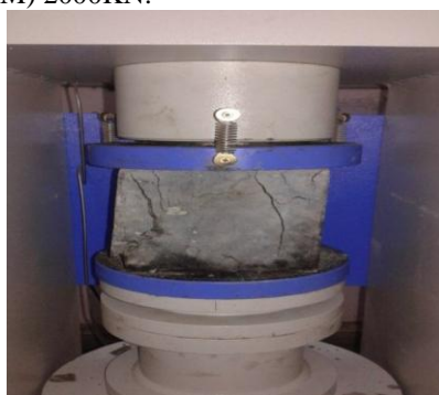
Figure 3: Compression testing of cube
