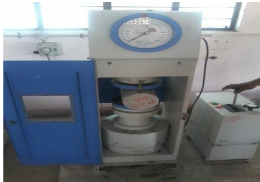
Figure 5: Split tensile testing of cylinder
