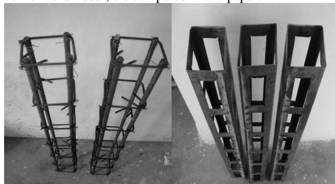
Figure 1: Rebar reinforcement and Prefabricated Cage System
