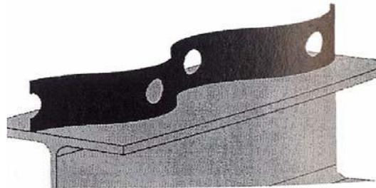
Figure 1.3: Oscillating Perfobond strip
