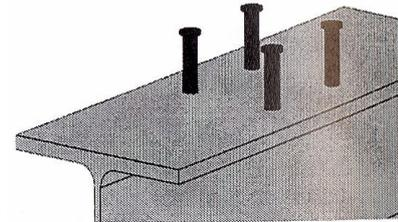
Figure 1.2: Headed Stud Connector
