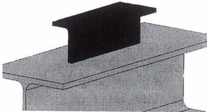
Figure 1.1: T-Shaped Shear connector
