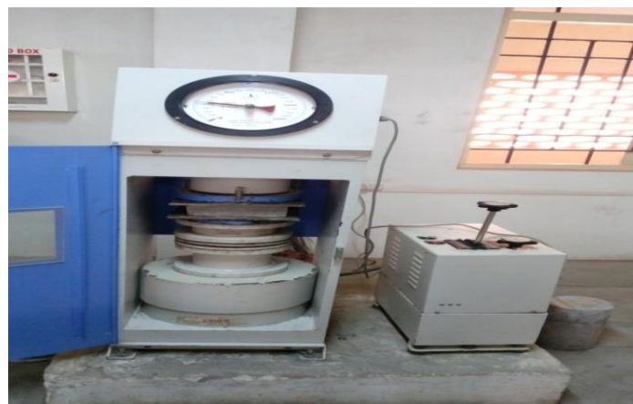
Figure 2: Compressive Strength Test
