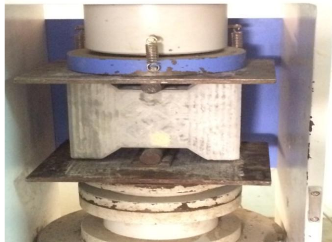
Figure 4: Split Tensile Strength Test
