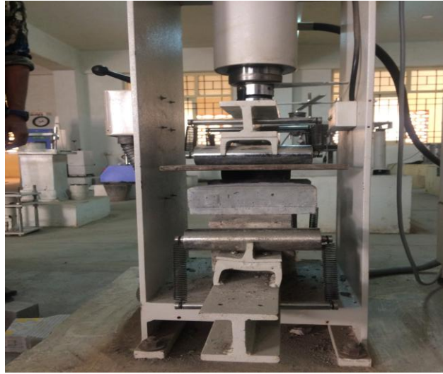
Figure 6: Flexural Strength Test
