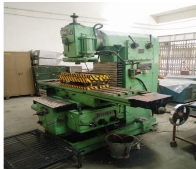
Figure 1: Friction Stir Welding Setup
