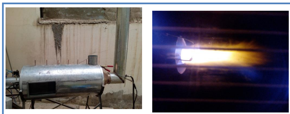
Figure 3: Air blast atomizer burner (left): Flame sample of alternative fuel (right)
